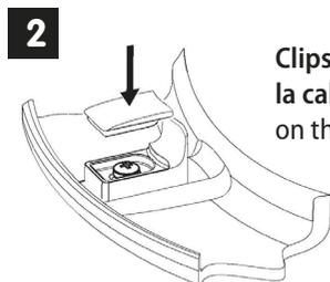
**Clipser le cache sur la cale / Clip the cover on the blocked buffer**
